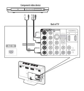
3 Connect an audio cable to the L and R audio jacks below the corresponding COMPONENT IN jacks and to the COMPONENT OUT AUDIO jacks on the component video device.
